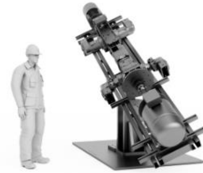
Set-up for functional testing with variable installation ( \pm 30^\circ on two planes)
